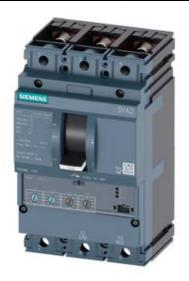
CIRCUIT BREAKER 3VA2 IEC FRAME 160 BREAKING CAPACITY CLASS C ICU=110KA @ 415 V 3POLE, LINE PROTECTION ETU350, LSI, IN=160A OVERLOAD PROTECTION IR=64A ...160A SHORT CIRCUIT PROTECTION ISD=1,5... 10 X IR, II=10 X IN BUSBAR CONNECTION
