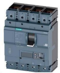
CIRCUIT BREAKER 3VA2 IEC FRAME 400 BREAKING CAPACITY CLASS H ICU=85KA @ 415 V 4-POLE, LINE PROTECTION ETU850, LSI, IN=250A OVERLOAD PROTECTION IR=100A ...250A SHORT CIRCUIT PROTECTION ISD=0,6..10X IN, II=1,5..12X IN NEUTRAL PROTECTION ADJUSTABLE (OFF, UPTO 160%) BUSBAR CONNECTION
