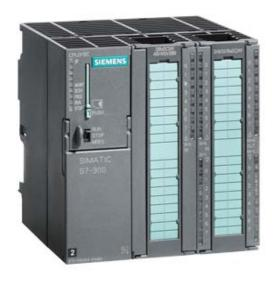
SIMATIC S7-300, CPU 313C, COMPACT CPU WITH MPI, 24 DI/16 DO, 4AI, 2AO 1 PT100, 3 FAST COUNTERS (30 KHZ), INTEGRATED 24V DC POWER SUPPLY, 128 KBYTE WORKING MEMORY, FRONT CONNECTOR (2 X 40PIN) AND MICRO MEMORY CARD REQUIRED
