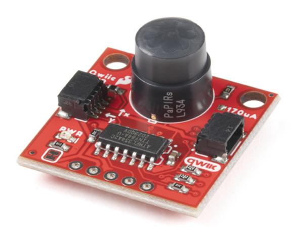
Passive Infrared (PIR) sensors are great for detecting motion in a small area around the sensor. The 170 $\mu$ A SparkFun EKMC4607112K Qwiic PIR uses an EKM-series PIR sensor from Panasonic® paired with an ATTiny84 to interact with it using I²C with the Qwiic system. The EKM-series PIR sensors are optimized for small movements to offer motion-sensing options for continuously powered applications.
