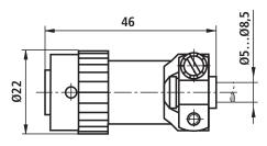
Plug-in connector, separate order stating Material no. **R901043330**
