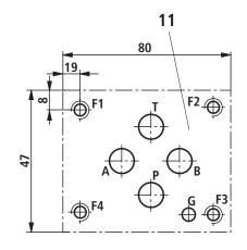
**Subplates** according to data sheet RE 45052 (separate order)
