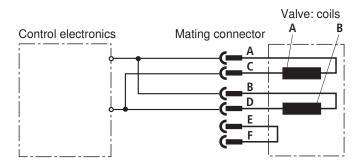
The coils are connected in parallel in the mating connector or on the amplifier (see figure).
