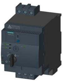
SIRIUS, COMPACT STARTER, REVERSING STARTER 690 V, 24 V AC/DC, 50 ... 60 HZ, 3 ... 12 A, IP20, MAIN CIRCUIT CONNECTION: SCREW TERMINAL, AUXILIARY CIRCUIT CONNECTION: PLUG-IN, W/O TERMINALS
