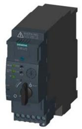
SIRIUS, COMPACT STARTER, DIRECT STARTER . 690 V, 24 V DC,  $0.32 \dots 1.25$  A, IP20, CONN. MAIN CIRCUIT: PLUG-IN, W/O TERMINALS, CONN. CONTROL CIRCUIT: SCREW TERMINAL
