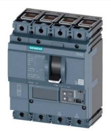
CIRCUIT BREAKER 3VA2 IEC FRAME 160 BREAKING CAPACITY CLASS C ICU=110KA @ 415 V 4POLE, LINE PROTECTION ETU550, LSI, IN=25A OVERLOAD PROTECTION IR=10A ...25A SHORT CIRCUIT PROTECTION ISD=0,6..10X IN, II=1,5..12X IN NEUTRAL PROTECTION ADJUSTABLE (OFF, UPTO 160%) CABLE CONNECTION
