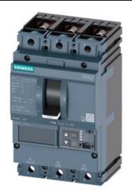
CIRCUIT BREAKER 3VA2 IEC FRAME 250 BREAKING CAPACITY CLASS M ICU=55KA @ 415 V 3POLE, LINE PROTECTION ETU550, LSI, IN=250A OVERLOAD PROTECTION IR=100A ...250A SHORT CIRCUIT PROTECTION ISD=0,6..10X IN, II=1,5..10X IN NEUTRAL PROTECTION OPTIONAL WITH EXT. CT,UPTO 160% BUSBAR CONNECTION
