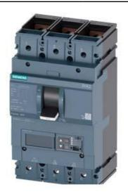
CIRCUIT BREAKER 3VA2 IEC FRAME 400 BREAKING CAPACITY CLASS H ICU=85KA @ 415 V 3-POLE, LINE PROTECTION ETU560, LSIG, IN=250A OVERLOAD PROTECTION IR=100A ...250A SHORT CIRCUIT PROTECTION ISD=0,6..10X IN, II=1,5..12X IN NEUTRAL PROTECTION OPTIONAL WITH EXT. CT;UPTO 160% GROUND-FAULT, SWITCHABLE IG=0,2... 1 X IN, TG=0,05-0,8MS BUSBAR CONNECTION
