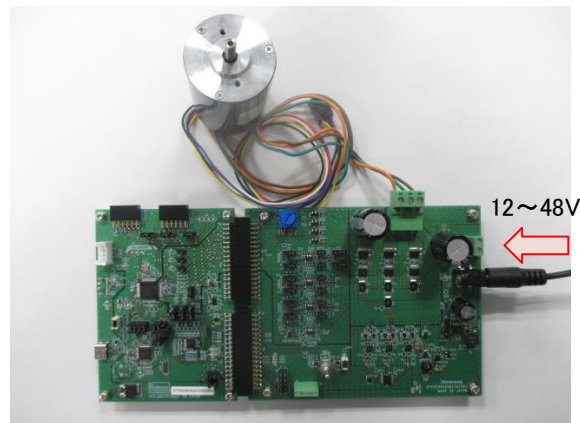
Figure 4-10 Power supply from DC jack
