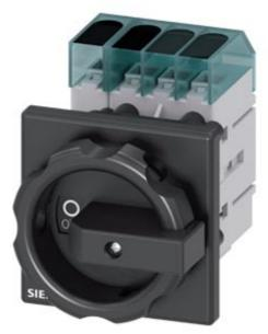
Load disconnector 3LD3, lu 63 A Main switch 3-pole + N Rated operating capacity at AC-23 A at 400V 22.0 kW Front plate mounting Basic switch with Central hole mounting 22.5mm Toggle drive black 66x66 mm
