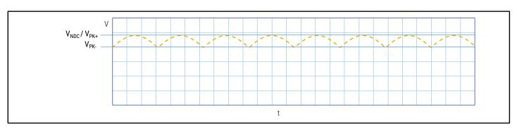
The applied peak-to-peak ripple voltage shall not exceed 0.1 x  $V_{NDC}$ . The peak voltage shall not exceed the rated voltage  $V_{NDC}$ .
