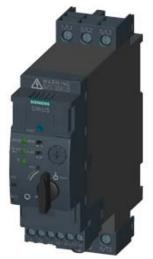
SIRIUS, COMPACT STARTER, DIRECT STARTER. 690 V, 24 V DC, 0.1 ... 0.4 A, IP20, CONN. MAIN CIRCUIT: SCREW TERMINAL, CONN. CONTROL CIRCUIT: SCREW TERMINAL
