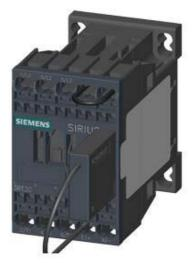
CONT. F. RAILW. A., AC-3, 5.5KW 400V, DC 110V, 0,7...1,25\*US, VARISTOR INTEGRATED, 3POL,SZ S00, STANDING BUILT-IN SPRING-LOADED TERMINAL
