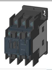
CONTACTOR, AC-3, 18.5KW/400V, 1NO+1NC, AC 110V 50HZ, 120V 60HZ 3-POLE, SZ S0 RING CABLE LUG CONNECTION
