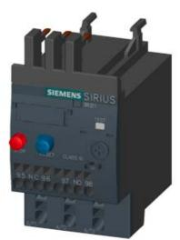
OVERLOAD RELAY 3.5...5.0 A FOR MOTOR PROTECTION SZ S00, CLASS 10, F. MOUNTING ONTO CONTACTOR MAIN CIRCUIT: SPRING TERMINAL AUX. CIRCUIT: SPRING TERMINAL MANUAL-AUTOMATIC-RESET
