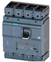
CIRCUIT BREAKER 3VA2 IEC FRAME 400 BREAKING CAPACITY CLASS C ICU=110KA @ 415 V 4-POLE, LINE PROTECTION ETU320, LI, IN=250A OVERLOAD PROTECTION IR=100A ...250A SHORT CIRCUIT PROTECTION II=12 X IN NEUTRAL PROTECTION ADJUSTABLE(OFF,50%,100%) BUSBAR CONNECTION
