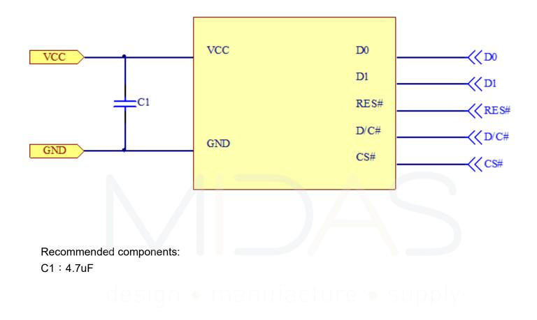
Note: The capacitor value is recommended value. Select appropriate value against module application.
