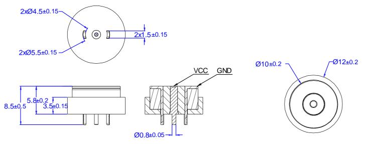
RECOMMEND PCB LAYOUT Layout Tolerance: ± 0.05mm
