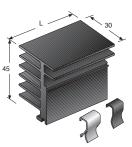
High power dissipation, extruded heatsinks designed to accommodate one or more TO220 packages via a clip retaining feature (clips available separately). Shaped to minimise board space, with a threaded slot provided to aid assembly. Choice of thermal resistance.
