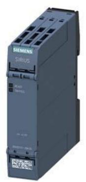
Thermistor motor prot. relay Standard evaluation unit 22.5 mm enclosure Spring-type terminals 2 CO contacts US = 24 V AC/DC Auto RESET Suitable for bimetal switches 2 LEDs (READY/TRIPPED) Galvanic separation
