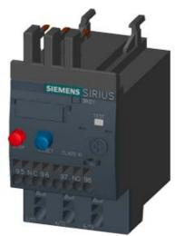
OVERLOAD RELAY 5.5...8.0 A FOR MOTOR PROTECTION SZ S00, CLASS 10, F. MOUNTING ONTO CONTACTOR MAIN CIRCUIT: SPRING TERMINAL AUX. CIRCUIT: SPRING TERMINAL MANUAL-AUTOMATIC-RESET
