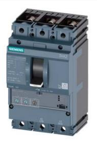
CIRCUIT BREAKER 3VA2 IEC FRAME 160 BREAKING CAPACITY CLASS M ICU=55KA @ 415 V 3POLE, LINE PROTECTION ETU320, LI, IN=40A OVERLOAD PROTECTION IR=16A ...40A SHORT CIRCUIT PROTECTION II=12 X IN BUSBAR CONNECTION
