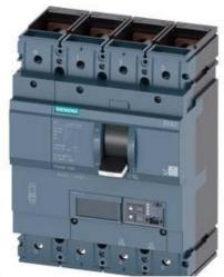
CIRCUIT BREAKER 3VA2 IEC FRAME 630 BREAKING CAPACITY CLASS C ICU=110KA @ 415 V 4-POLE, LINE PROTECTION ETU550, LSI, IN=500A OVERLOAD PROTECTION IR=200A ...500A SHORT CIRCUIT PROTECTION ISD=0,6..10X IN, II=1,5..14X IN NEUTRAL PROTECTION ADJUSTABLE (OFF, UPTO 100%) BUSBAR CONNECTION
