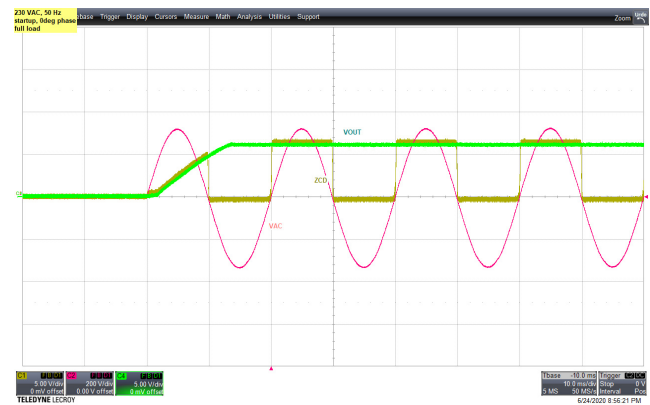
Figure 17 – 230 VAC 50 Hz, Full Load. CH1: ZCD, 5 V / div., 5 ms / div. CH2: V IN , 100 V / div., 5 ms / div. CH4: V OUT , 5 V / div., 5 ms / div.
