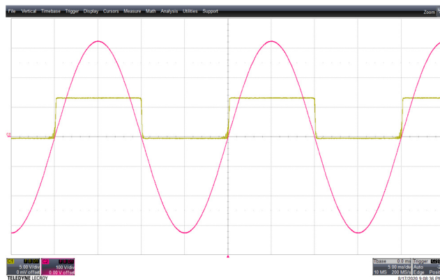
Figure 11 – 230 VAC 50 Hz. CH1: ZCD, 5 V / div., 5 ms / div. CH2: V_{IN} , 100 V / div., 5 ms / div.
