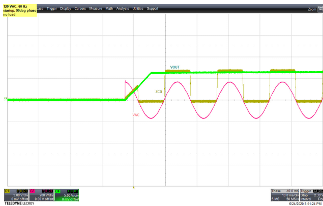
Figure 18 – 120 VAC 60 Hz, No-Load. CH1: ZCD, 5 V / div., 5 ms / div. CH2: V_{IN} , 100 V / div., 5 ms / div. CH4: V_{OUT} , 5 V / div., 5 ms / div.
