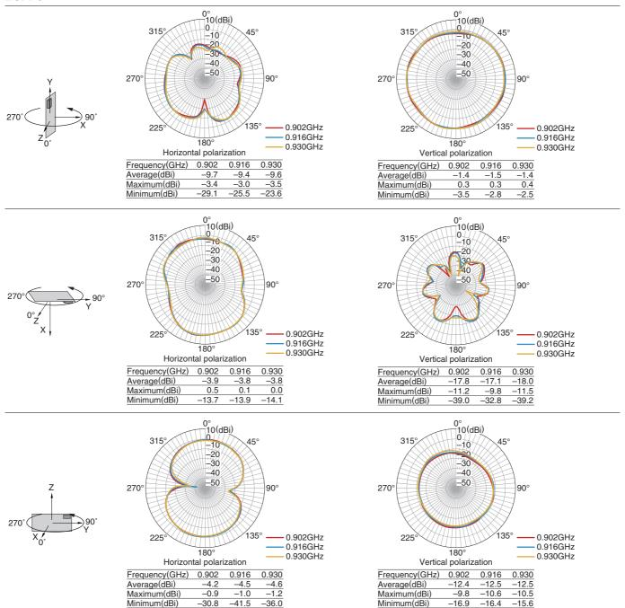
• Tested antenna has been soldered. Evaluation board size is 100x20x1mm.
