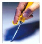
By designing the bit to wrap around the heating element, ANTEX have ensured maximum heat transfer into the bit, and minimum heat loss to ambient. Such is the efficiency that tests have proven that an ANTEX 25 watt iron has equivalent soldering power to many other manufacturers' 40 watt irons.
