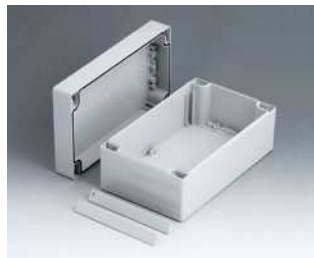
C2112202 ROBUST-BOX 120 BREIT, Ausf. II PC (UL 94 HB) lichtgrau RAL 7035 200x120x90mm IP 66
