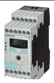
TEMPERATURUEBERWACHUNGSRELAIS PT100/1000, KTY83/84, NTC 3 FUEHLER, 2 SCHWELLW., DIGITAL -58 GRAD F BIS 932 GRAD F 24-240V AC/DC 2 X 1 W + 1 S, BAUBR. 45 MM SCHRAUBANSCHLUSS
