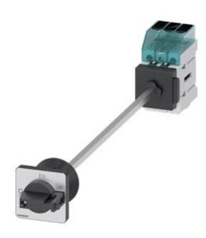
Switch disconnector 3LD3, main switch 3-polig, lu 32A operational switch at AC-23 A at 400 V 11,5 kW floor mounting Base mounting with door coupling center-hole 22,5 mm knob-operated mechanism black  $48 \times 48 \text{ mm}$
