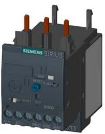
OVERLOAD RELAY 0.1...0.4 A FOR MOTOR PROTECTION SIZE S0, CLASS 20 CONTACTOR ASS. MAIN CIRCUIT: SCREW CONN. AUX.CIRCUIT: SCREW CONN. MANUAL-AUTOM.-RESET
