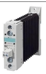
SEMI-COND. CONTACTOR 3RF2,1-PH. AC51 30 A 40 DEG. C 48-460 V / 24V DC LOW POWER SHORT CIRC. PROOF UP TO 25 A WITH B-AUTOMAT
