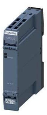
Thermistor motor prot. relay Compact evaluation unit 17.5 mm enclosure Spring-type terminals 1 CO contact US = 24 V AC/DC Auto RESET Suitable for bimetal switches Supply = output voltage 1 LED (READY)
