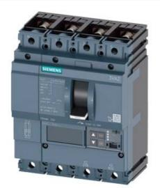
CIRCUIT BREAKER 3VA2 IEC FRAME 250 BREAKING CAPACITY CLASS C ICU=110KA @ 415 V 4POLE, LINE PROTECTION ETU550, LSI, IN=250A OVERLOAD PROTECTION IR=100A ...250A SHORT CIRCUIT PROTECTION ISD=0,6..10X IN, II=1,5..10X IN NEUTRAL PROTECTION ADJUSTABLE (OFF, UPTO 100%) BUSBAR CONNECTION
