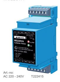
PTC-relay for the application as a protection device against inadmissible heating up at electrical equipment in areas with explosive gases (zones 1 and 2) and areas with combustible dust (21 an 22), e.g. for direct temperature-monitoring of explosion-proof motors EEx e and EEx d.
