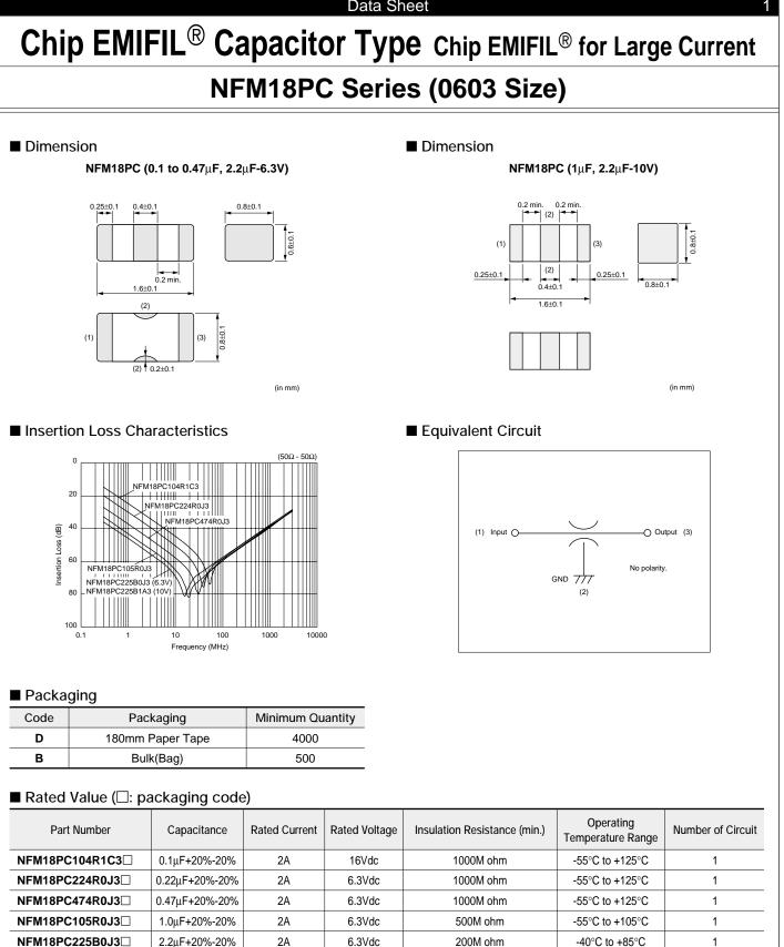
This data sheet is applied for CHIP EMIFIL<sup>®</sup> used for General Electronics equipment for your design.
