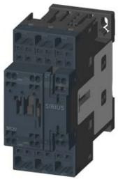
CONTACTOR, AC-3, 18.5KW/400V, 1NO+1NC, AC 24V 50/60HZ, 3-POLE, SZ S0 SPRING-LOADED TERMINAL
