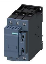
CONTACTOR, AC-6B, 75KVAR/400V, 2NC, 110V AC, 50HZ, 3-POLE, SIZE S2 SCREW TERMINAL
