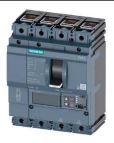
CIRCUIT BREAKER 3VA2 IEC FRAME 160 BREAKING CAPACITY CLASS L ICU=150KA @ 415 V 4POLE, LINE PROTECTION ETU860, LSIG, IN=63A OVERLOAD PROTECTION IR=25A ...63A SHORT CIRCUIT PROTECTION ISD=0,6..10X IN, II=1,5..12X IN NEUTRAL PROTECTION ADJUSTABLE (OFF, UPTO 160%) GROUNDFAULT, SWITCHABLE IG=0,2... 1 X IN, TG=0,050,8MS CABLE CONNECTION
