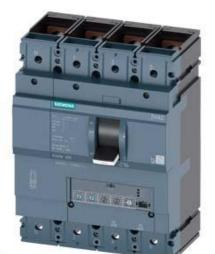
CIRCUIT BREAKER 3VA2 IEC FRAME 400 BREAKING CAPACITY CLASS M ICU=55KA @ 415 V 4-POLE, LINE PROTECTION ETU350, LSI, IN=400A OVERLOAD PROTECTION IR=160A ...400A SHORT CIRCUIT PROTECTION ISD=1,5... 10 X IR, II=10 X IN NEUTRAL PROTECTION ADJUSTABLE(OFF,50%,100%) BUSBAR CONNECTION
