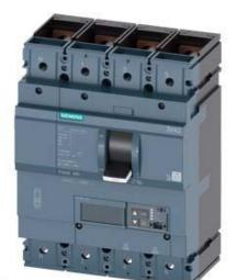
CIRCUIT BREAKER 3VA2 IEC FRAME 400 BREAKING CAPACITY CLASS C ICU=110KA @ 415 V 4-POLE, LINE PROTECTION ETU560, LSIG, IN=400A OVERLOAD PROTECTION IR=160A ...400A SHORT CIRCUIT PROTECTION ISD=0,6..10X IN, II=1,5..10X IN NEUTRAL PROTECTION ADJUSTABLE (OFF, UPTO 100%) GROUND-FAULT, SWITCHABLE IG=0,2... 1 X IN, TG=0,05-0,8MS BUSBAR CONNECTION
