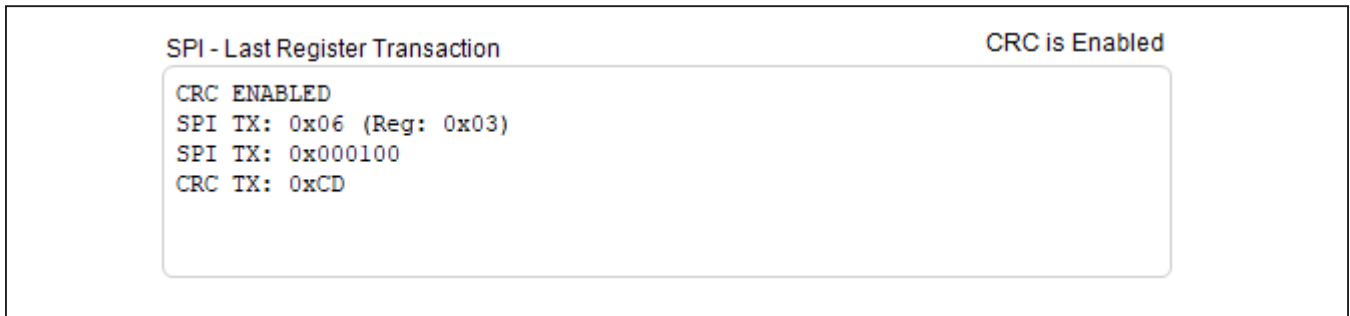
Figure 6. SPI Write Transaction with CRC Enabled
