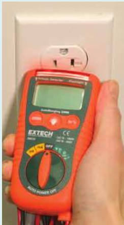
Built-in Non-Contact Voltage Detector. Red LED bar lights when live wire detected.
