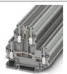
Disconnect terminal block, With test socket screws for insertion of test plugs, Connection type: Screw connection, Cross section: 0.14 mm² - 4 mm², AWG: 26 - 12, Width: 5.2 mm, Color: gray, Mounting type: NS 35/7,5, NS 35/15
