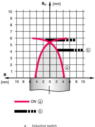
a Inductive switchb Standard measuring plate
