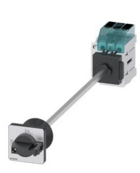
Switch disconnector 3LD3, main switch 3-polig, lu 16A operational switch at AC-23 A at 400 V 7,5 kW floor mounting Base mounting with door coupling center-hole 22,5 mm knob-operated mechanism black 48 x 48 mm with auxiliary 1NO+1NC
