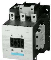
CONTACTOR, 55KW/400V/AC-3, AC(40...60HZ)/DC OPERATION UC 200...277V AUXIL. CONTACTS 2NO+2NC 3-POLE, SIZE S6 BAR CONNECTIONS ELECTRONIC OPERATING MECHANISM WITH PLC INTERFACE 24V DC SCREW TERMINAL
