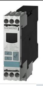
DIGITAL MONITORING RELAY COS-PHI A. CURRENT MONITORING FROM 90 TO 690V AC OVERSHOOT AND UNDERSHOOT INTERNAL POWER SUPPLY AC 50 TO 60 HZ SPIKE DELAY 0.1 TO 20S HYSTERESIS W. (I) 0.1 TO 2A 2 CHANGEOVER CONTACTS W. OR W/O ERROR LOG SCREW TERMINAL REPLACEMENT PRODUCT F. 3UG3014
