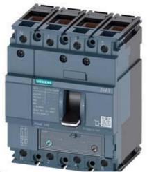
CIRCUIT BREAKER 3VA1 IEC FRAME 160 BREAKING CAPACITY CLASS H ICU=70KA @ 415 V 4-POLE, LINE PROTECTION TM240, ATAM, IN=50A OVERLOAD PROTECTION IR=35A ...50A SHORT CIRCUIT PROTECTION II=5...10 X IN NEUTRAL PROTECTION 100% CABLE CONNECTION
